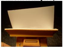
Parts 11 and 12 are the sides to the top of the clock and attach to part 10. When gluing the top to the bottom, it's easier to line things up from the back of the clock:
